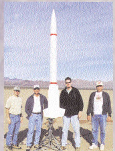
Brent McNeely and launch crew prepare the Stinger 98 for flight on the new M1315W at the Tripoli Vegas Turkey Shoot '98 launch. The Stinger flew to an altitude of 7,913 ft. and was recovered for a successful level three certification.
