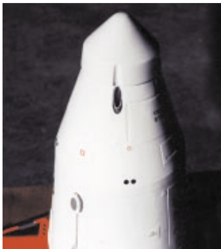
Detail view of internal launch lug.
