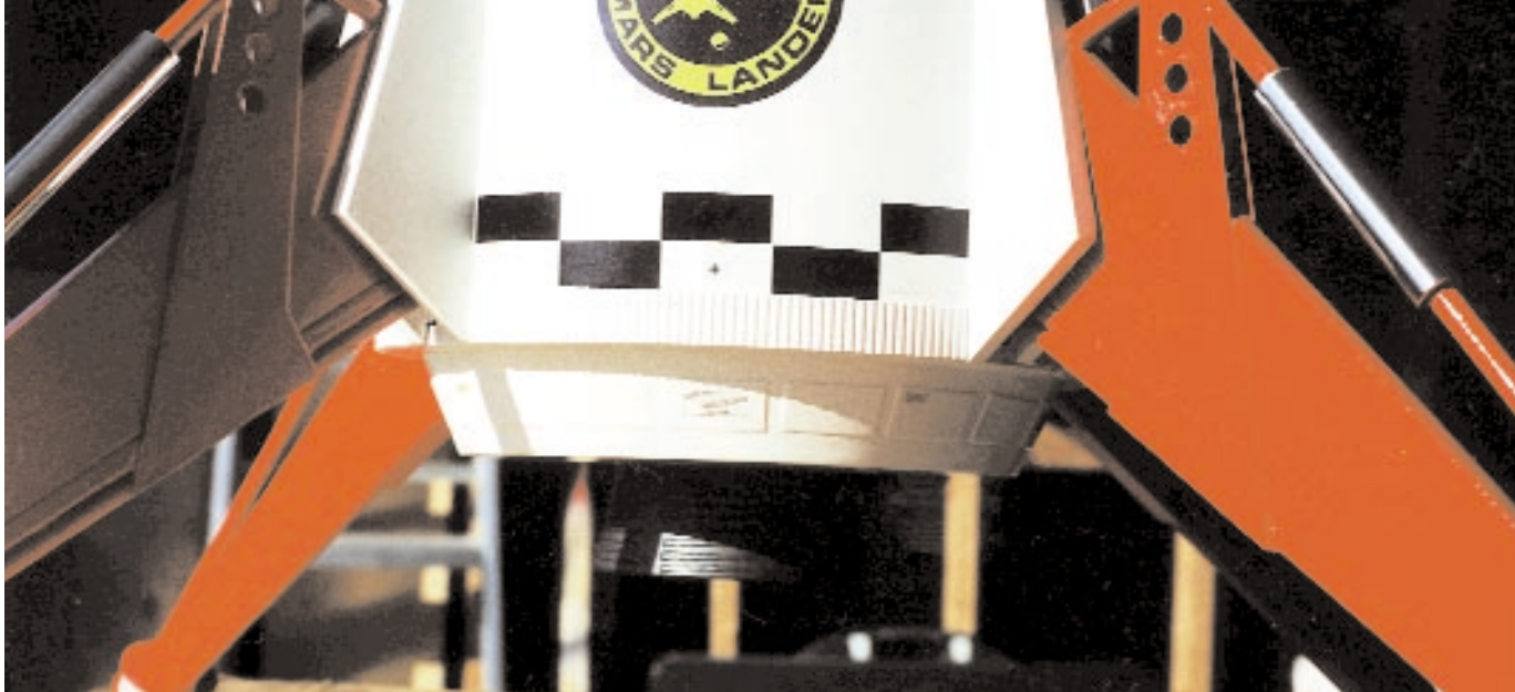
Detail view of the lower body. The nozzle also functions as the motor retainer.
