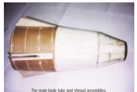
The main body tube and shroud assemblies.
