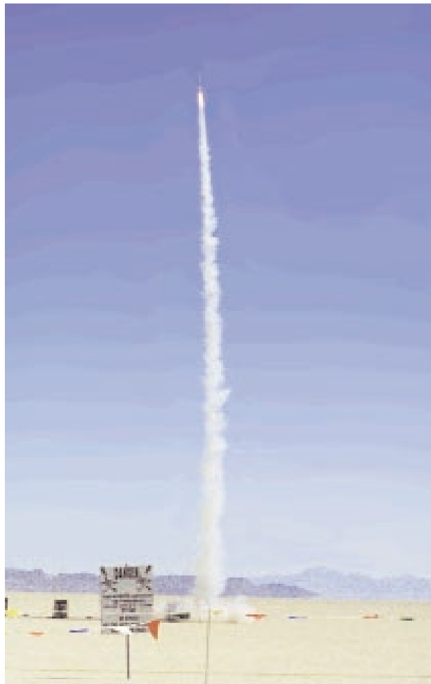
Launch of the "H" powered record flight to 8363 ft. on an AeroTech H-123W at the Back Rock Desert in June of 1999. The simulation showed it reaching 1,000 m.p.h.
