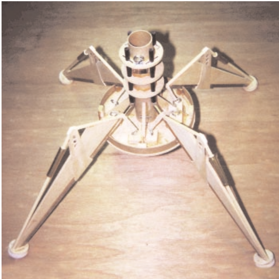
The assembled base unit showing the motor tube, base plate, and lander legs
