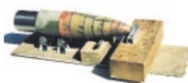
Neck alignment using rollers & fixed indexes.
