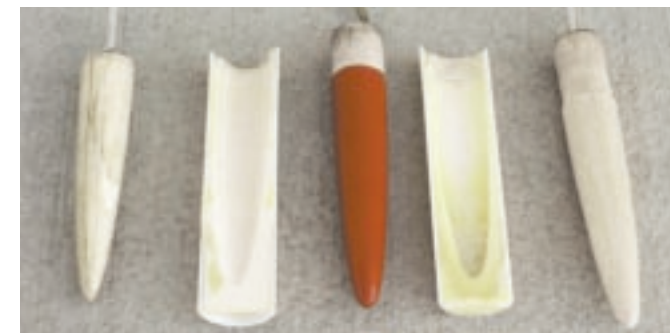
New 29mm elliptical nosecone for "F" TROOP-2 in middle; internal plug on left; mold halves on either side; moldmaking plug on right. Neck was attached using rod centering ring technique.
