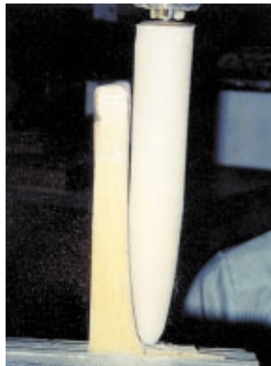
Contoured sanding block in cross slide vise taking the blank down closer to the final shape.
