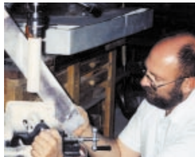
The diameter being brought down with the "heavy sanding tool" in the cross-slide vise (photo: Jeanne Hoover)
