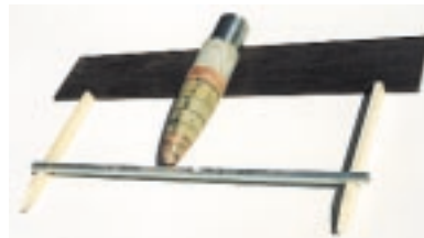
Neck alignment using board & straight edge.
