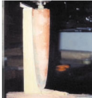
The dark areas are the low spots (dark orange on the right). Additional bondo will be applied there and re-sanded.
