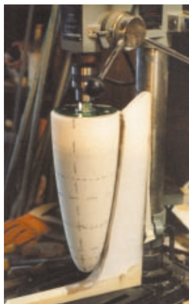
Black dotted lines will be the edges of the fiberglass strips. Blue dashed lines mark edges of the staggered second layer of fiberglass strips.
