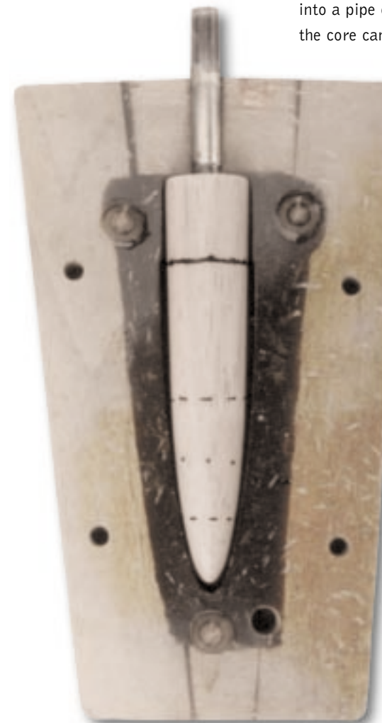
Here you see the fit of the male mold and female mold half. The space between will be filled with the laminate. The width of the crack will be the thickness of the wall.
