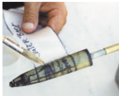
Core being fiberglassed using the wet lay-up process. (Photo: Hoover)
